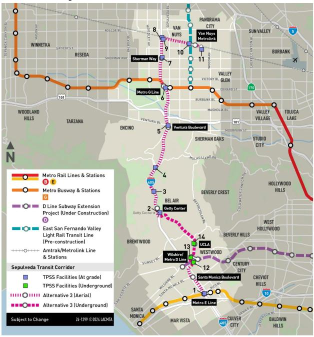
Figure 7-7. Alternative 3: Traction Power Substation Locations
