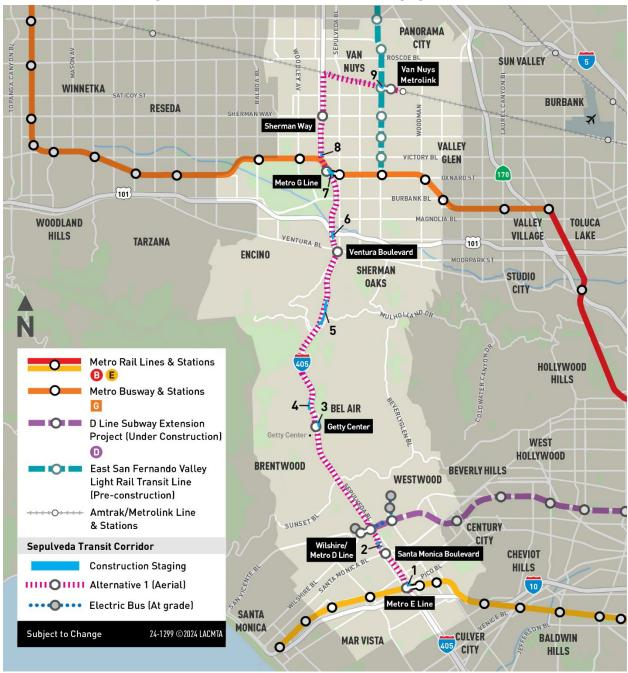
Figure 6-9. Alternative 1: Construction Staging Locations
