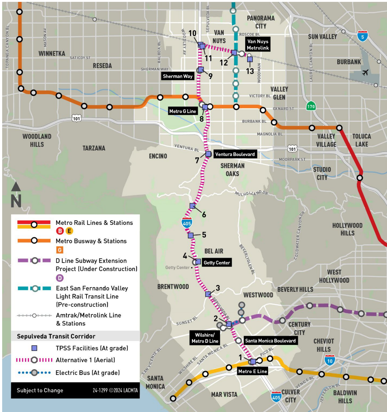
Figure 6-7. Alternative 1: Traction Power Substation Locations
