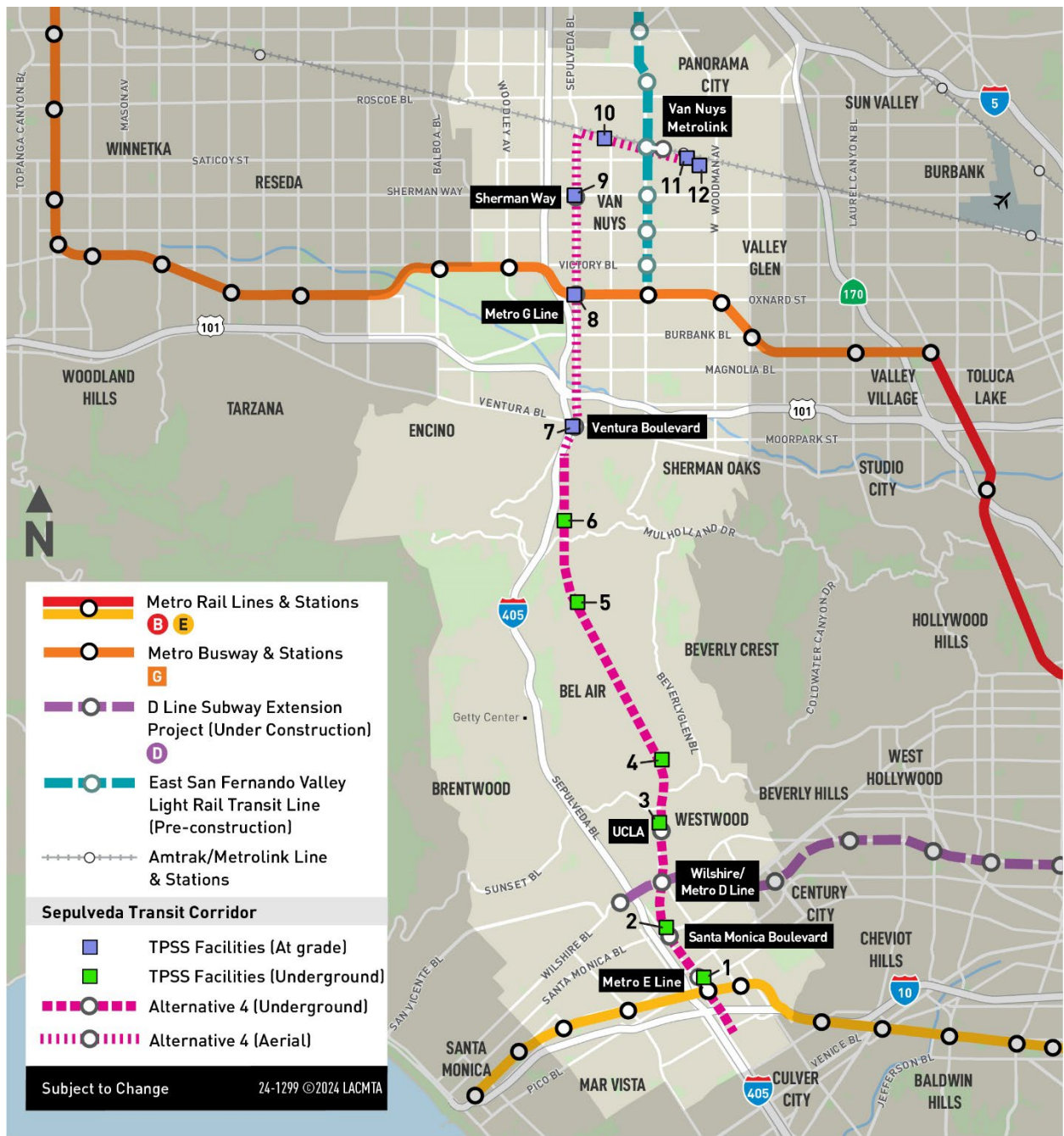
Figure 8-6. Alternative 4: Traction Power Substation Locations
