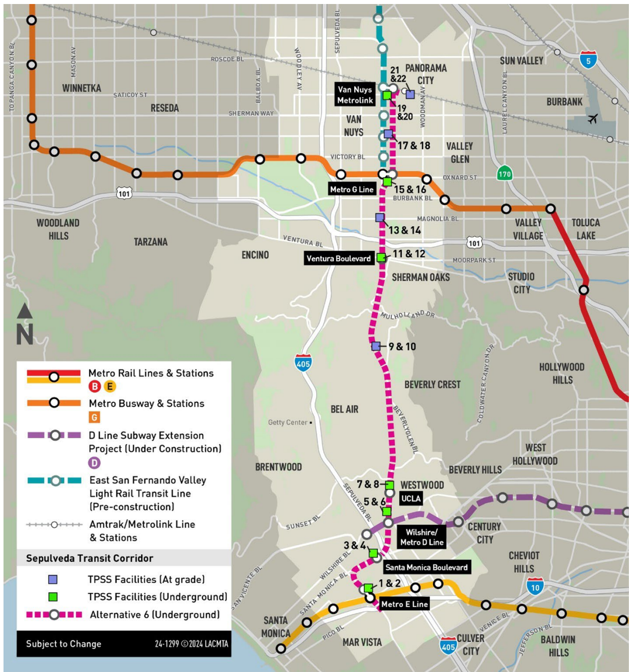
Figure 10-4. Alternative 6: Traction Power Substation Locations
