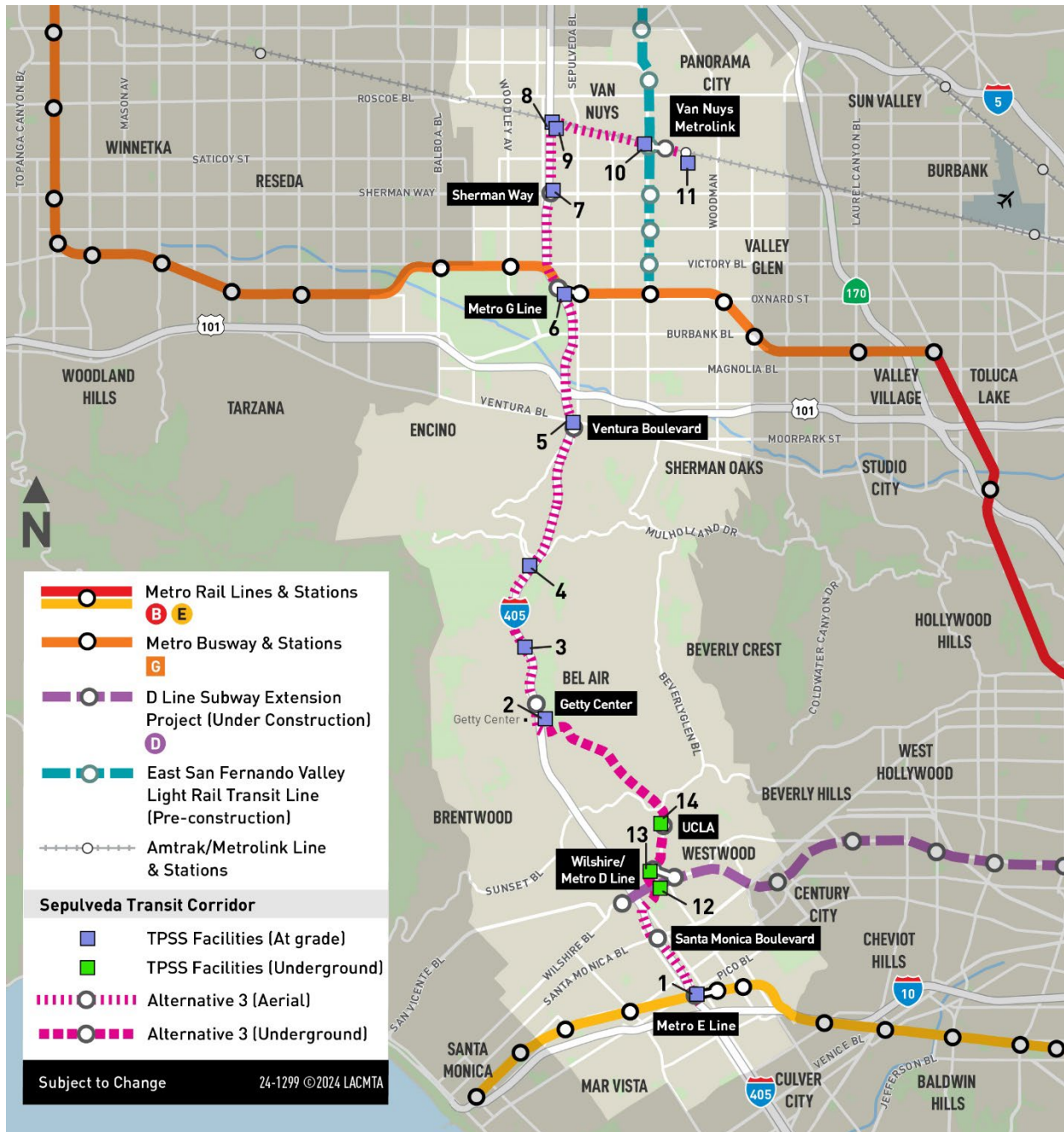
Figure 7-7. Alternative 3: Traction Power Substation Locations
