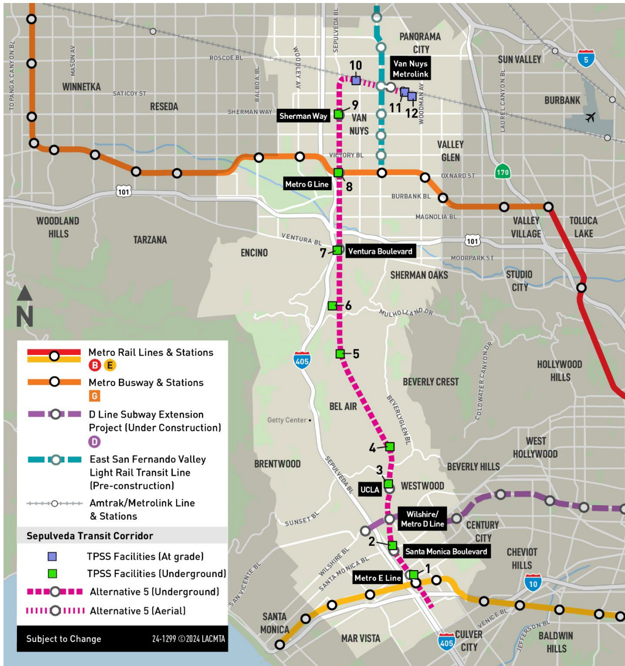
Figure 9-5. Alternative 5: Traction Power Substation Locations
