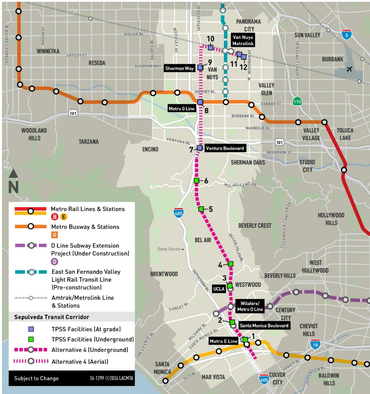
Figure 8-6. Alternative 4: Traction Power Substation Locations
