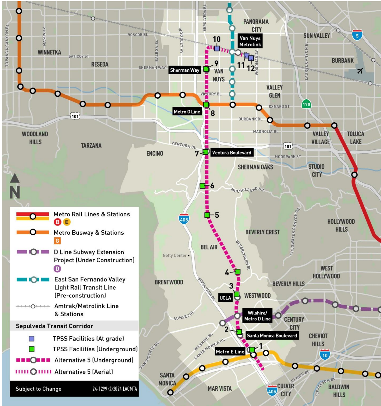
Figure 9-5. Alternative 5: Traction Power Substation Locations
