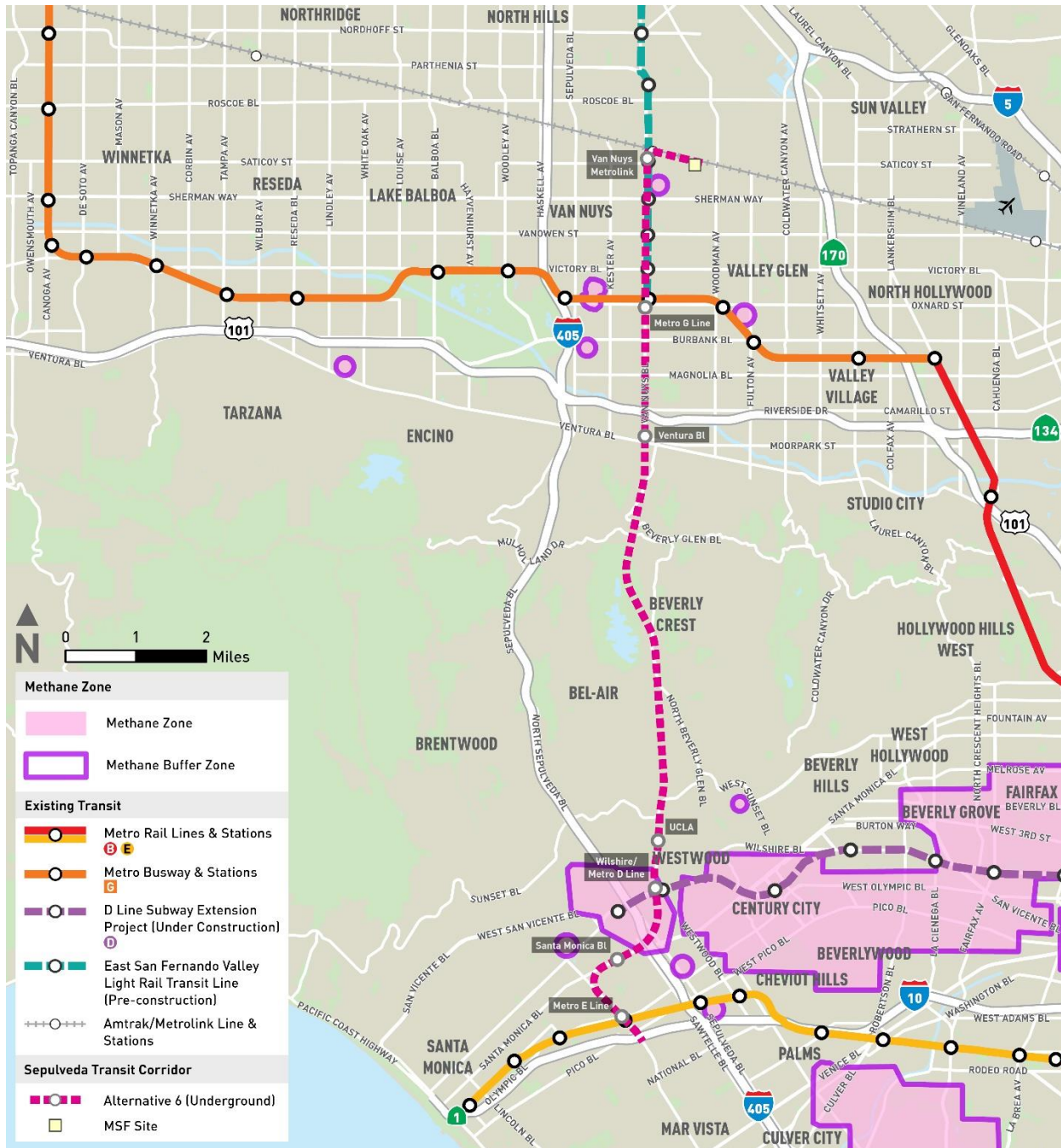
Figure 10-8. Alternative 6: Methane Hazard Zones
