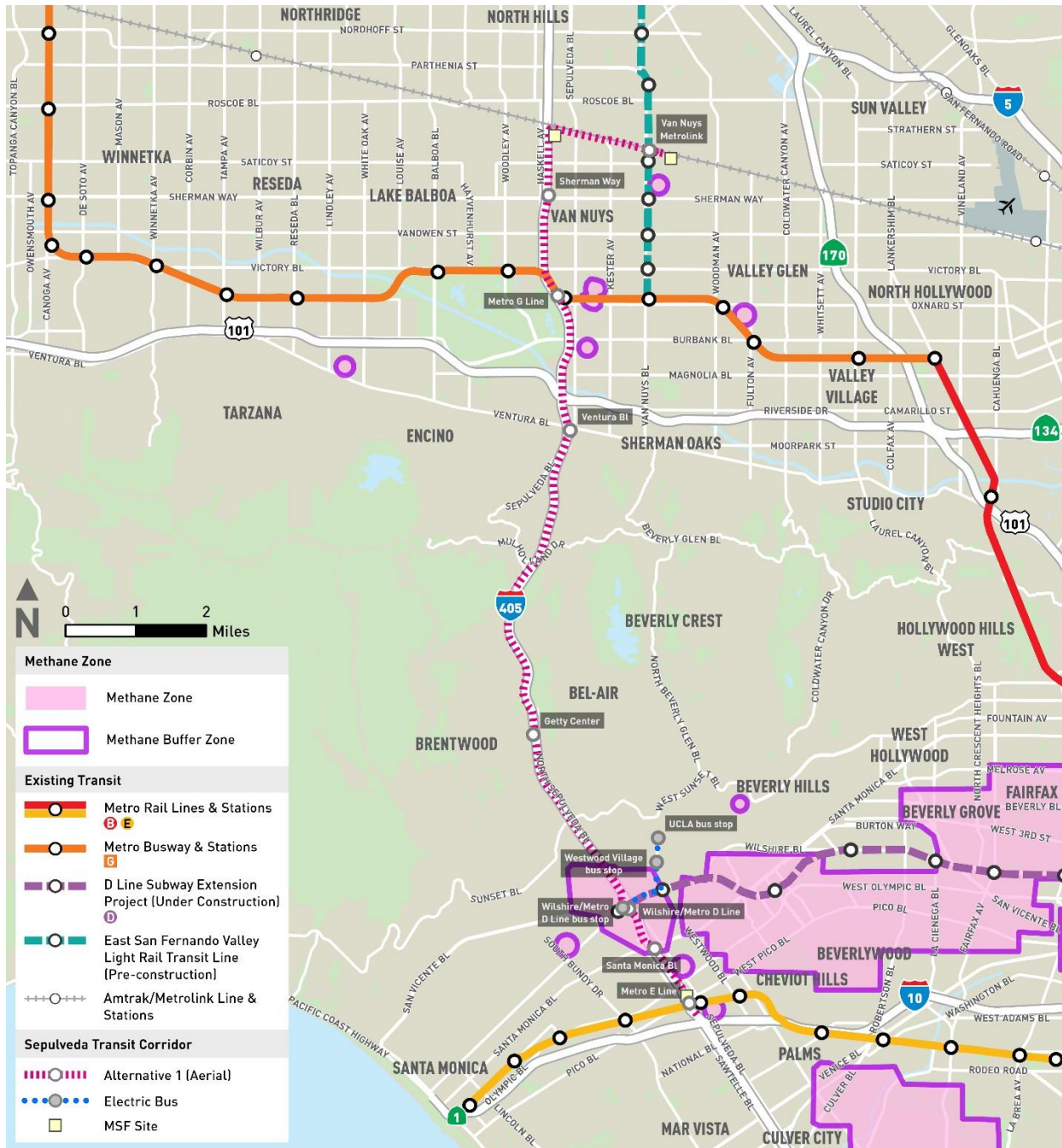
Figure 6-12. Alternative 1: Methane Hazard Zones
