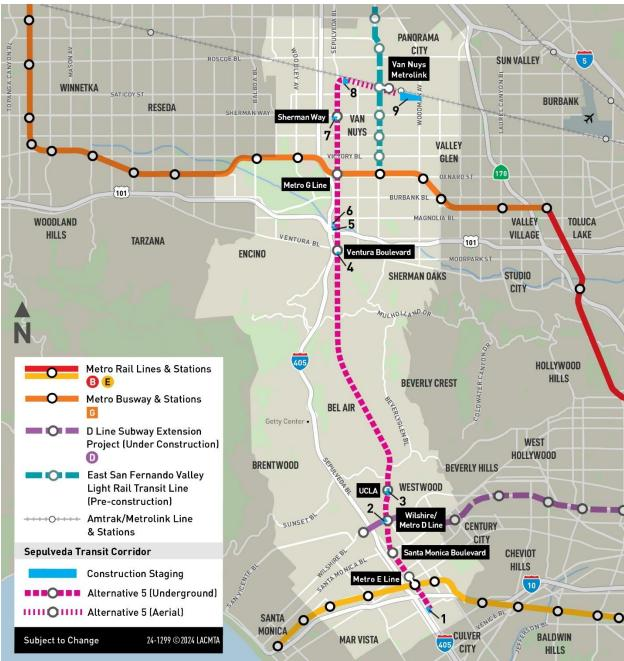
Figure 9-7. Alternative 5: On-Site Construction Staging Locations
