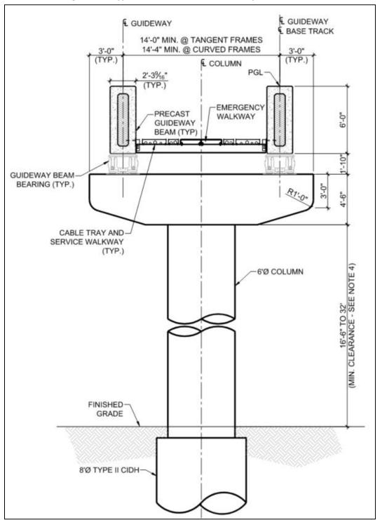
Figure 7-2. Typical Aerial Monorail Guideway Cross-Section
