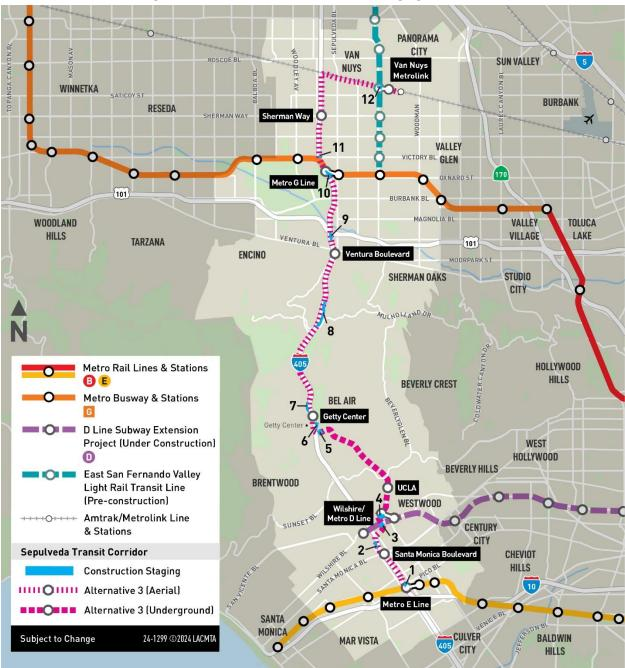
Figure 7-9. Alternative 3: Construction Staging Locations
