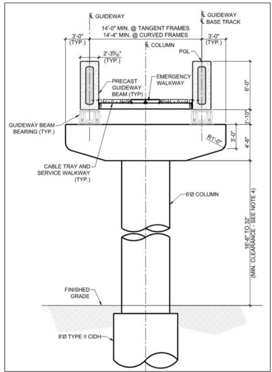
Figure 6-2. Typical Monorail Guideway Cross-Section
