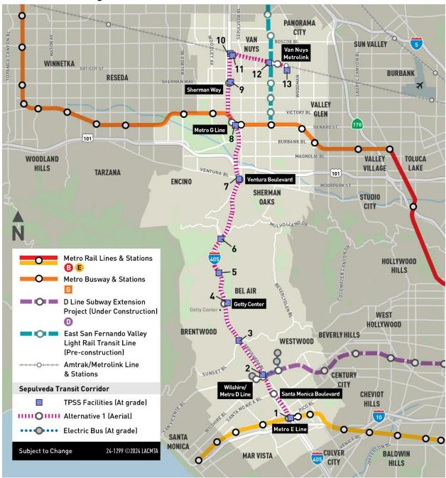
Figure 6-7. Alternative 1: Traction Power Substation Locations
