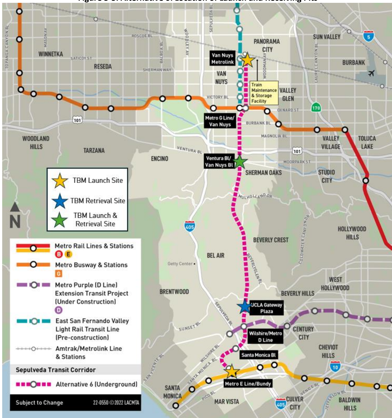
Figure 3-5. Alternative 6: Location of Launch and Receiving Pits
