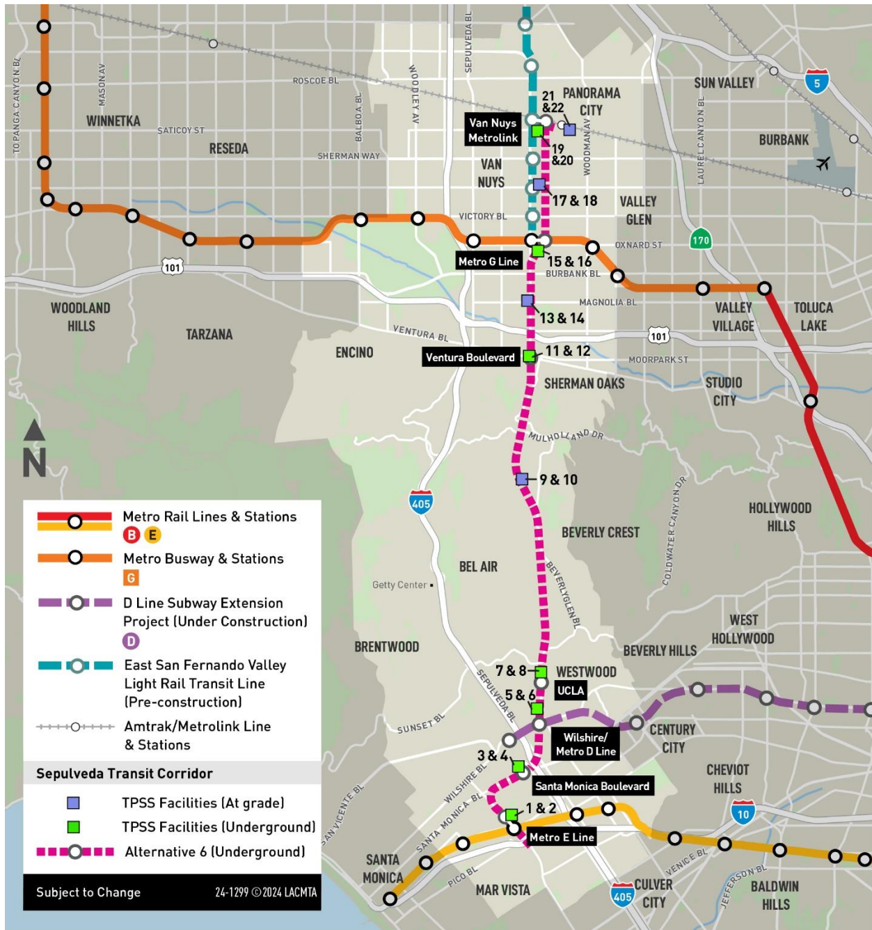
Figure 2-4. Alternative 6: Traction Power Substation Locations
