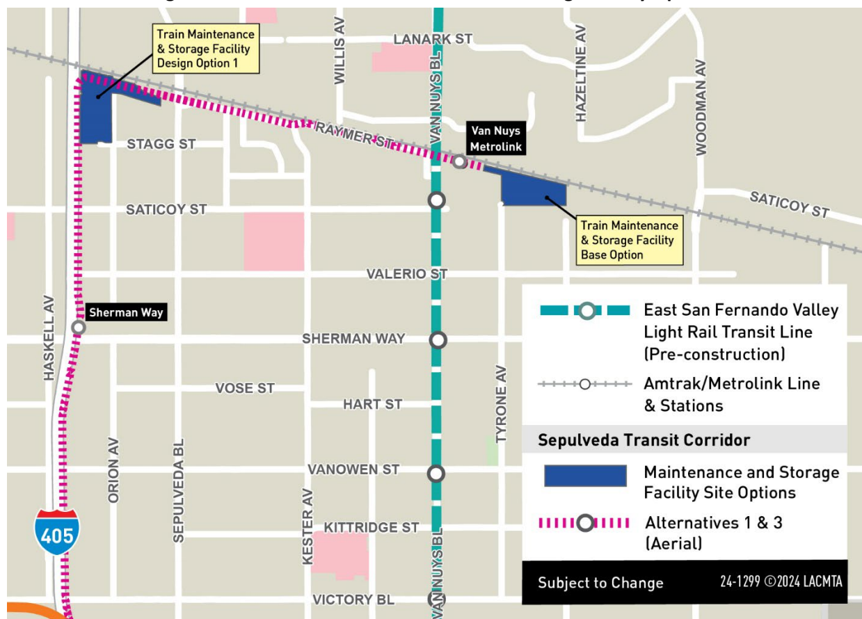
Figure 6-5. Alternative 1: Maintenance and Storage Facility Options
