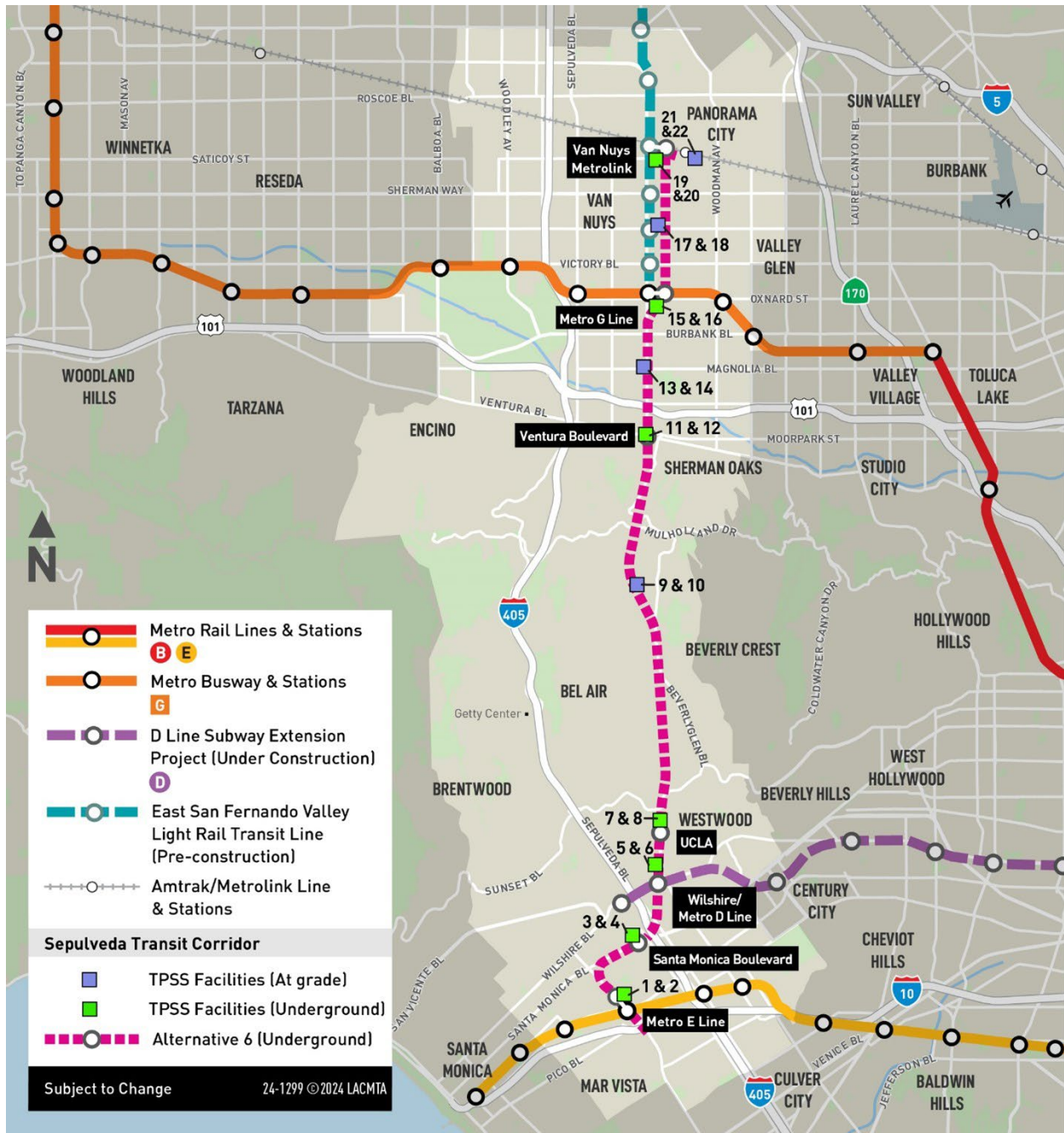
Figure 10-4. Alternative 6: Traction Power Substation Locations
