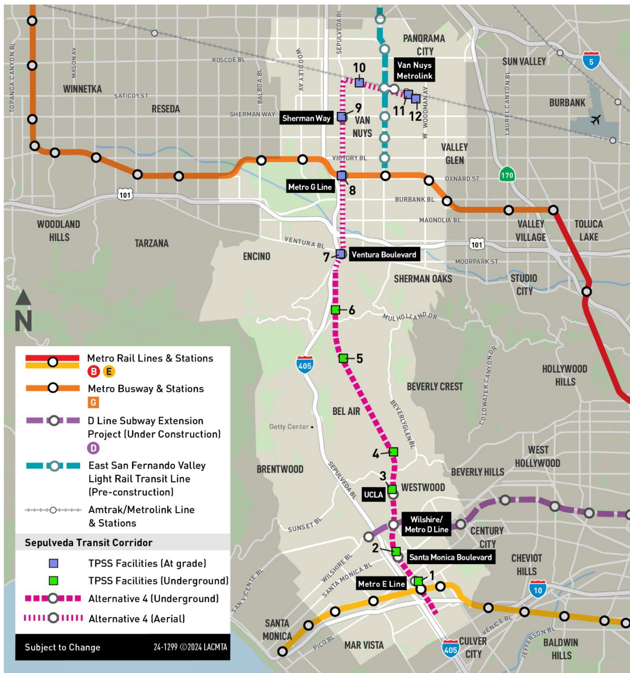
Figure 8-6. Alternative 4: Traction Power Substation Locations
