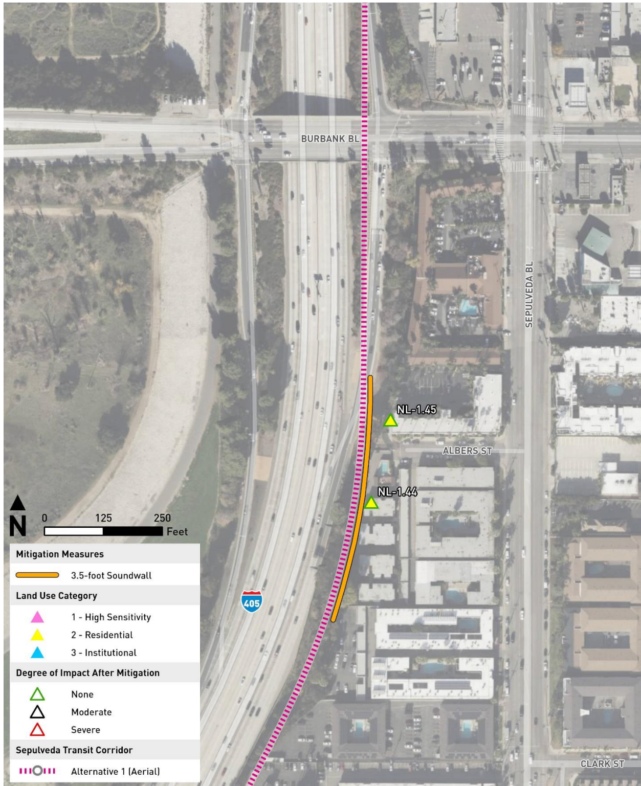
Figure 3.11-4. Alternative 1: Mitigated Rail Operations Noise Impacts – Magnolia Boulevard to Burbank Boulevard
