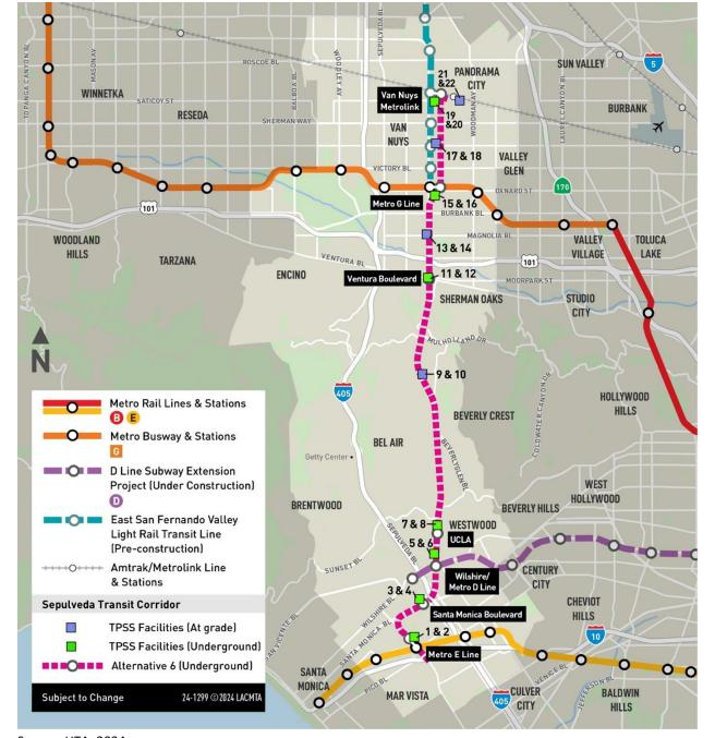
Figure 11-4. Alternative 6: Traction Power Substation Locations
