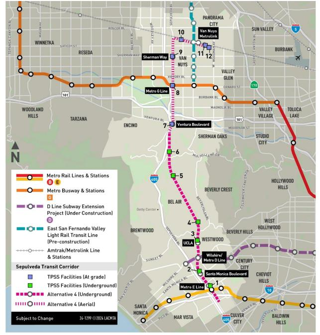
Figure 9-6. Alternative 4: Traction Power Substation Locations
