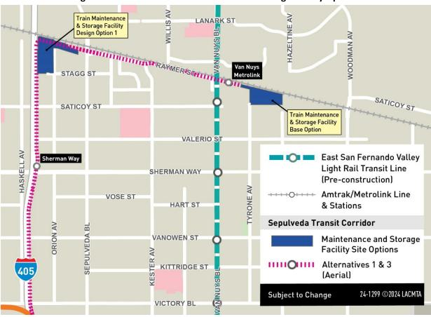
Figure 7-5. Alternative 1: Maintenance and Storage Facility Options
