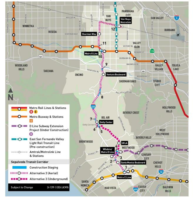
Figure 8-9. Alternative 3: Construction Staging Locations
