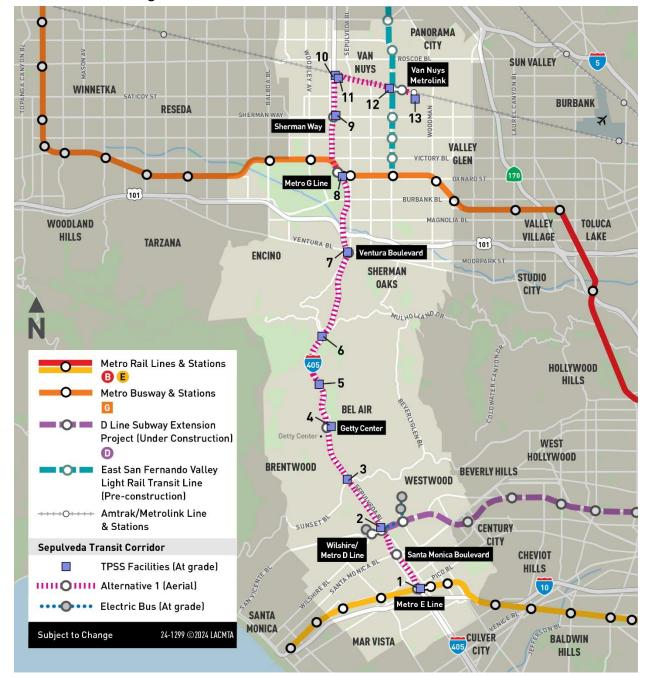
Figure 7-7. Alternative 1: Traction Power Substation Locations
