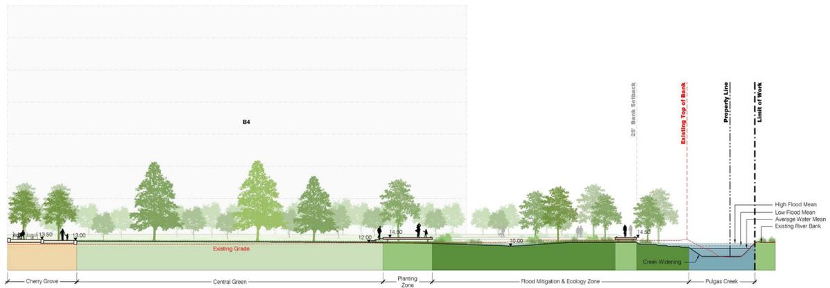
**Figure 22.4c: Conceptual Pulgas Creek Design Section 2**
