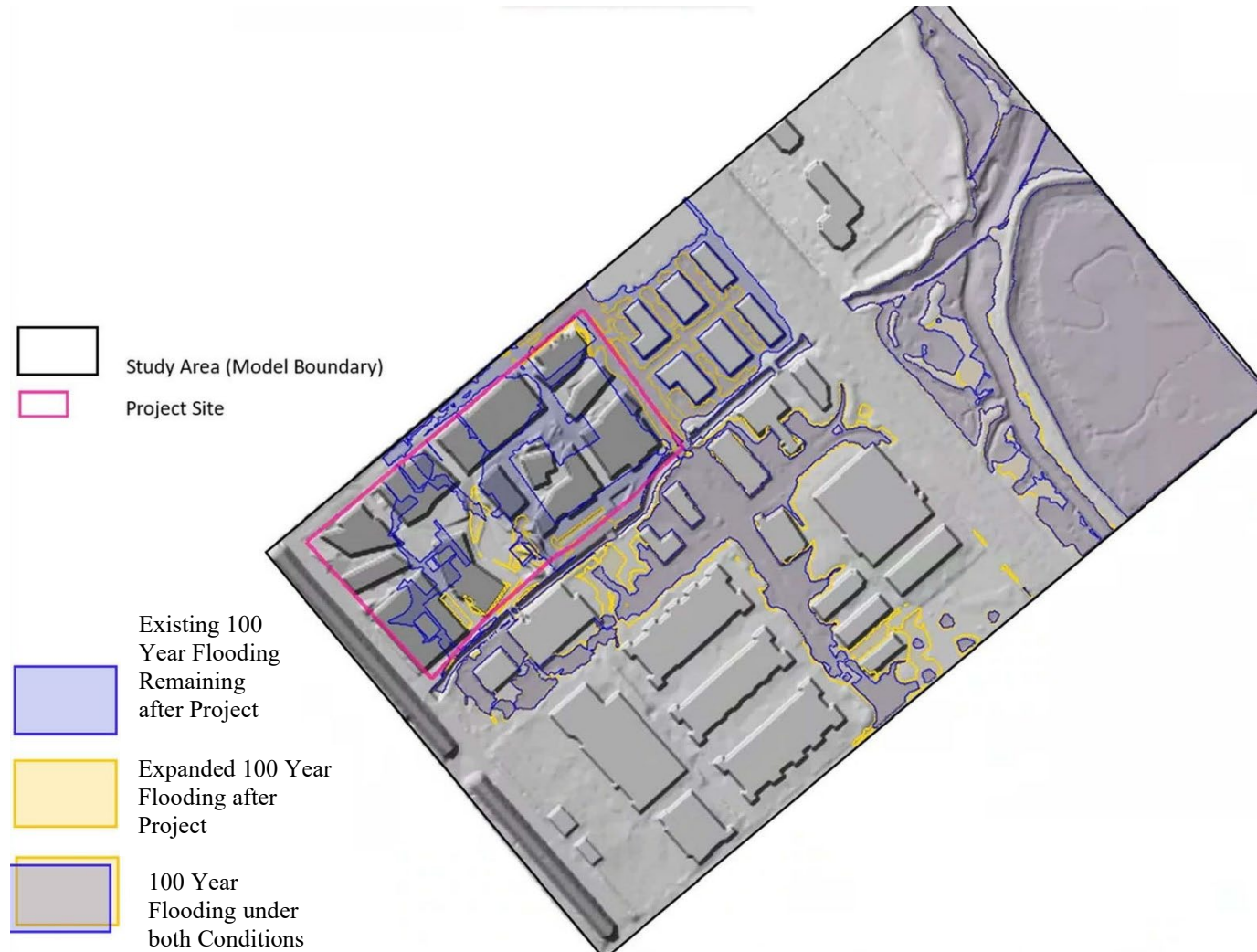
Figure 12.2: Overlay of Existing and Project with Original Design 100-Year Flood Extents Source: WRA, November 2020
