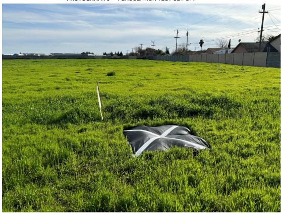
PHOTOGRAPH 10 - PERCOLATION TEST SET-UP.
