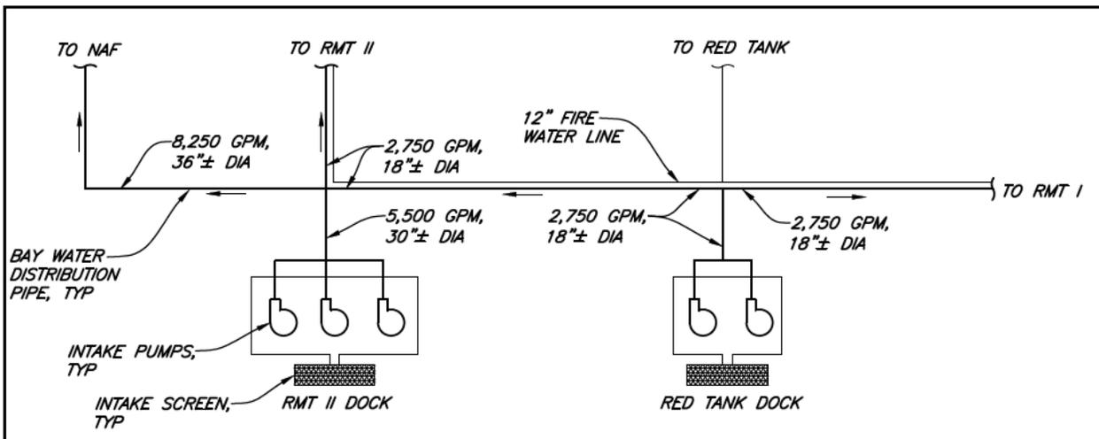
Image 2-19 Pipe Diameter and Volume of Water that Would Travel Through Different Sections of the Bay Water Line
