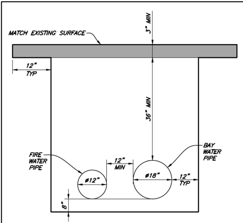
Image 2-20 Conceptual Trench Details in Areas Where the Bay Water Line and Fire Suppression Line Would Occur
