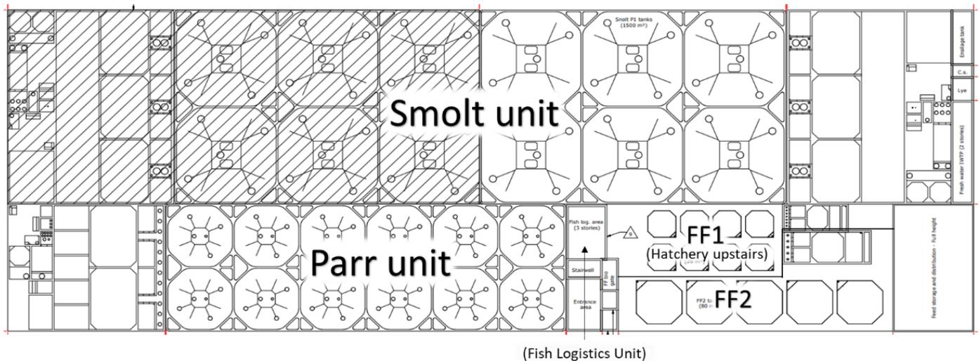
**Image 2-7**      **Layout of Tanks and RAS Systems in NAFC Hatchery Building**
