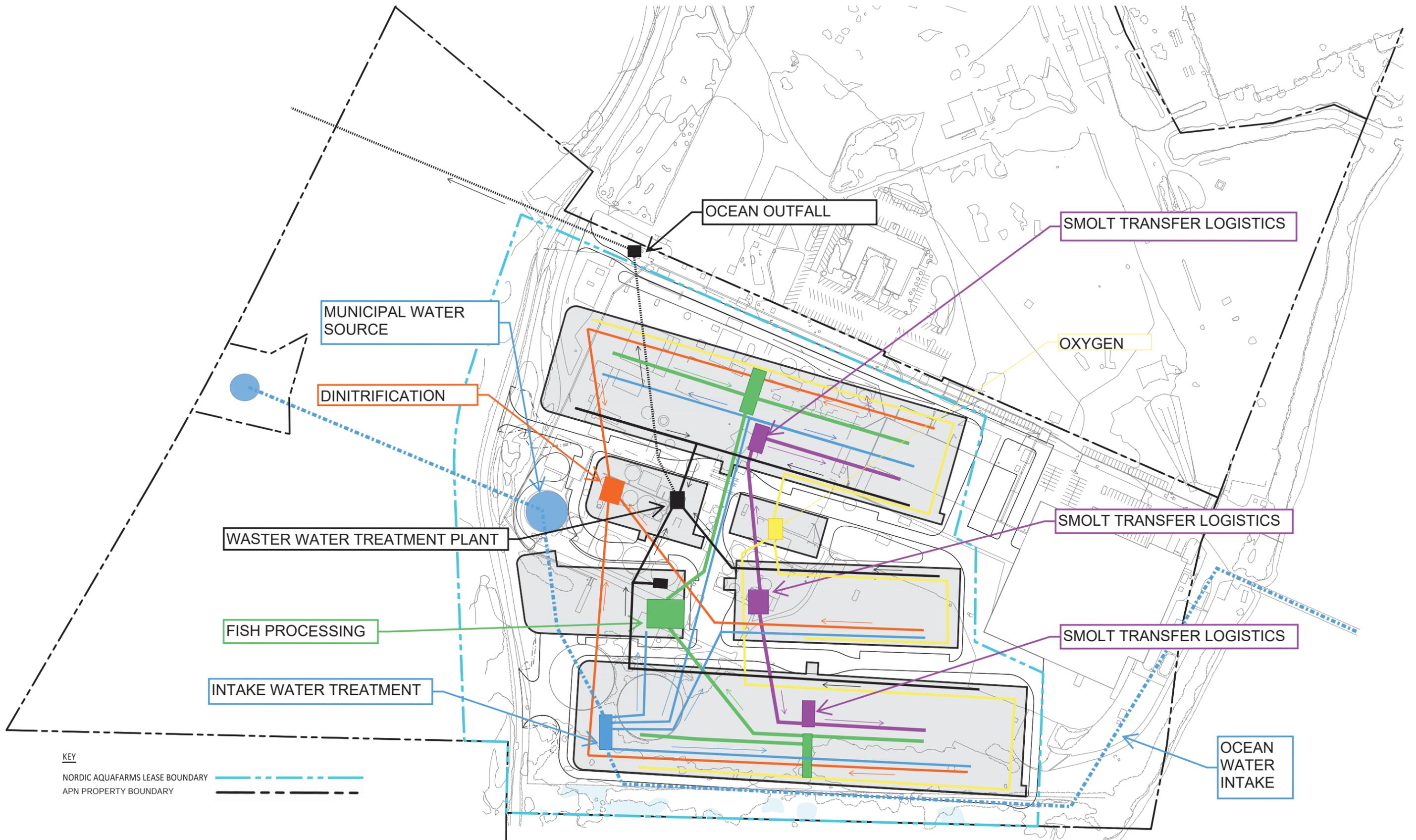
**Figure 2-12: CONCEPT PIPING LAYOUT**
