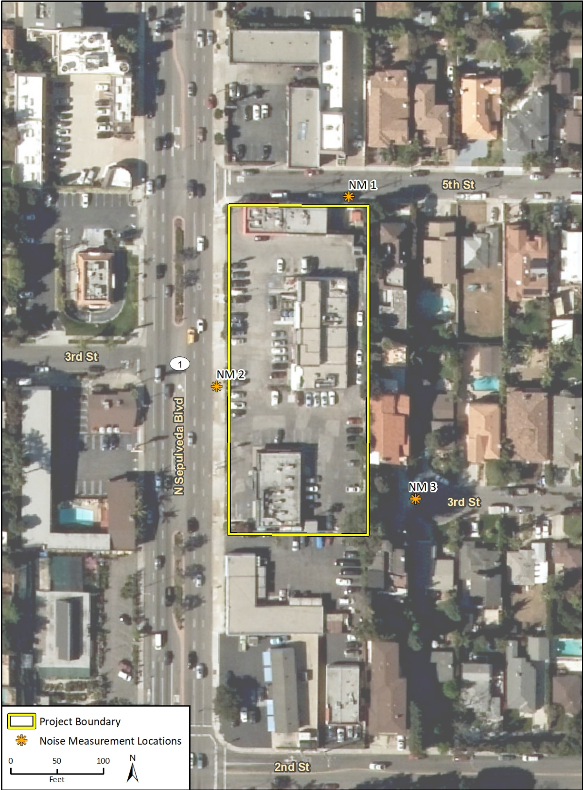
Figure 4.6-1 Sound Level Measurement and Sensitive Receiver Locations
