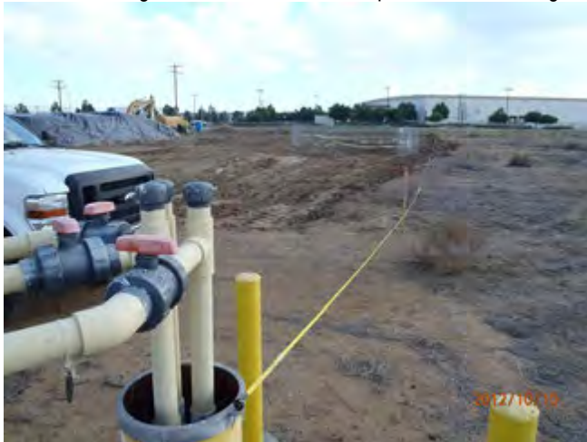
Looking South from 7SVE02 with measuring tape used to grid out site for confirmation sampling
