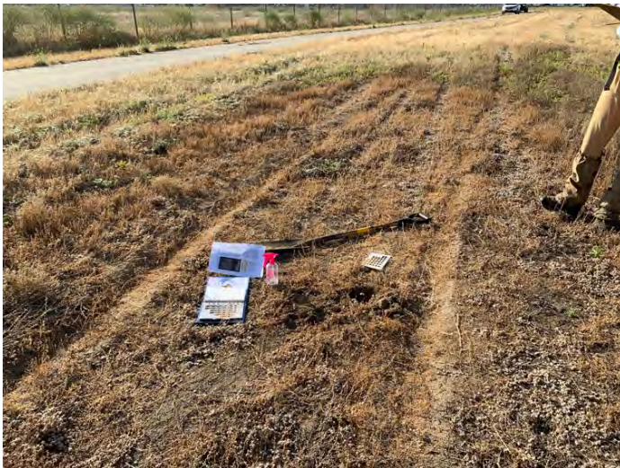
Photo 3. View of WDP 1, facing east. WDP 1 met the hydrophytic vegetation, hydric soil, and wetland hydrology parameters (33.876247, -117.250602).
