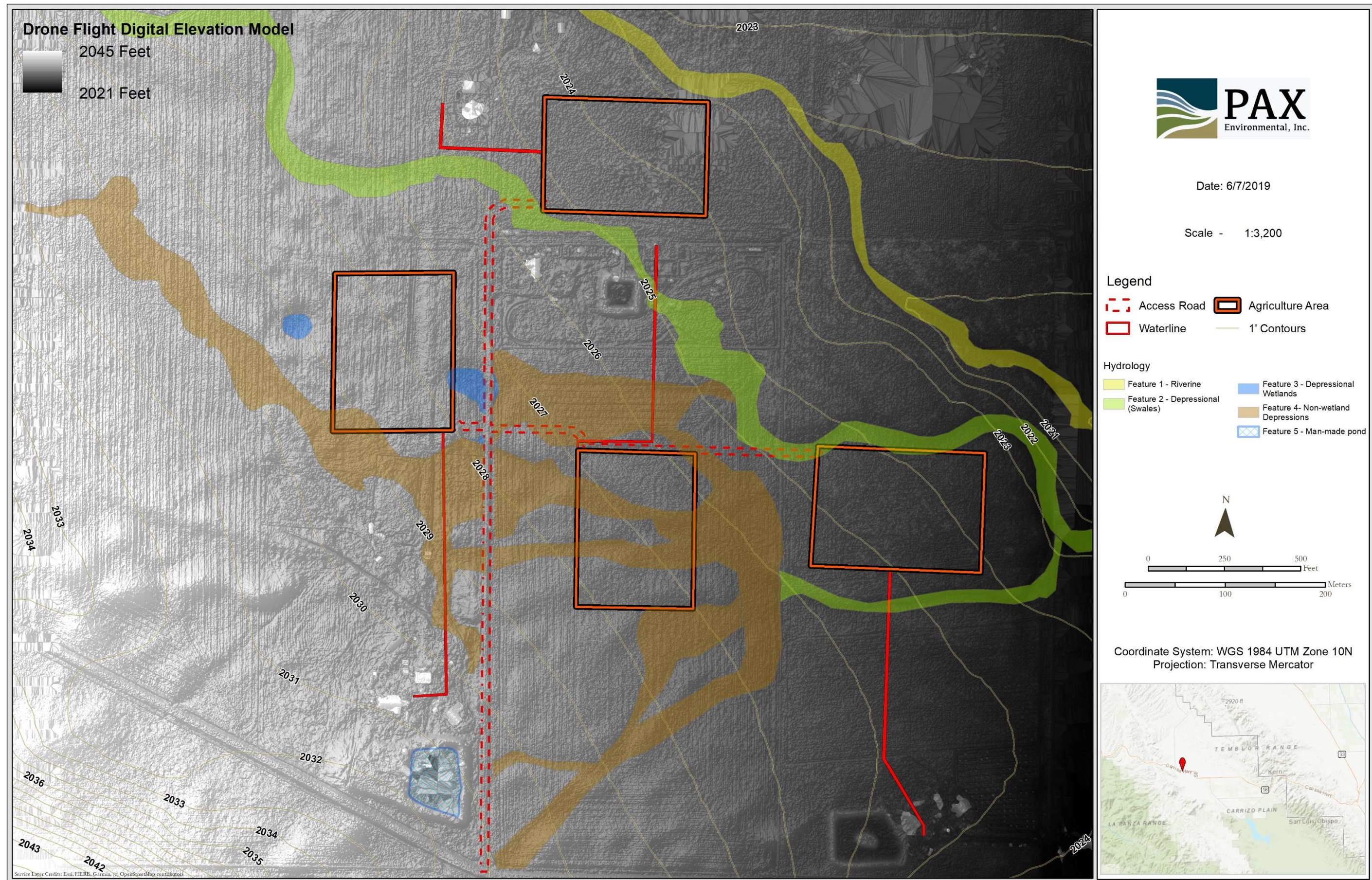
Figure 3: Drone flight topographic survey imagery with Project footprint and mapped hydrogeomorphic features.
