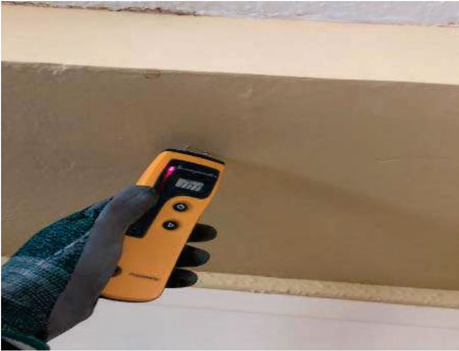
39. Marina Inn, Room 318 – View of elevated moisture reading on soffit.
