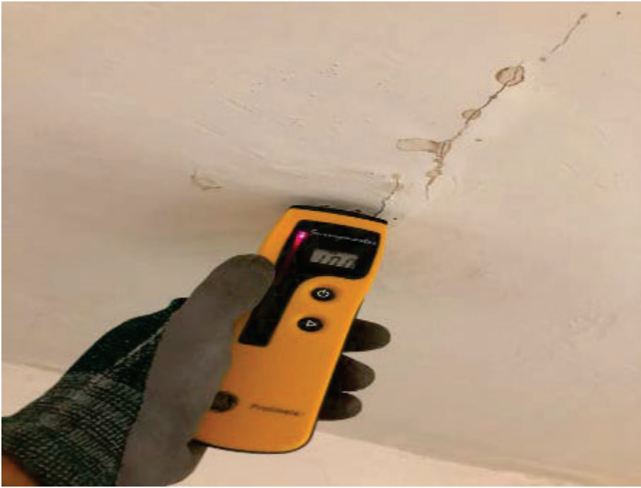
27. Marina Inn, Dana Point Room – View of elevated moisture readings on ceiling.
