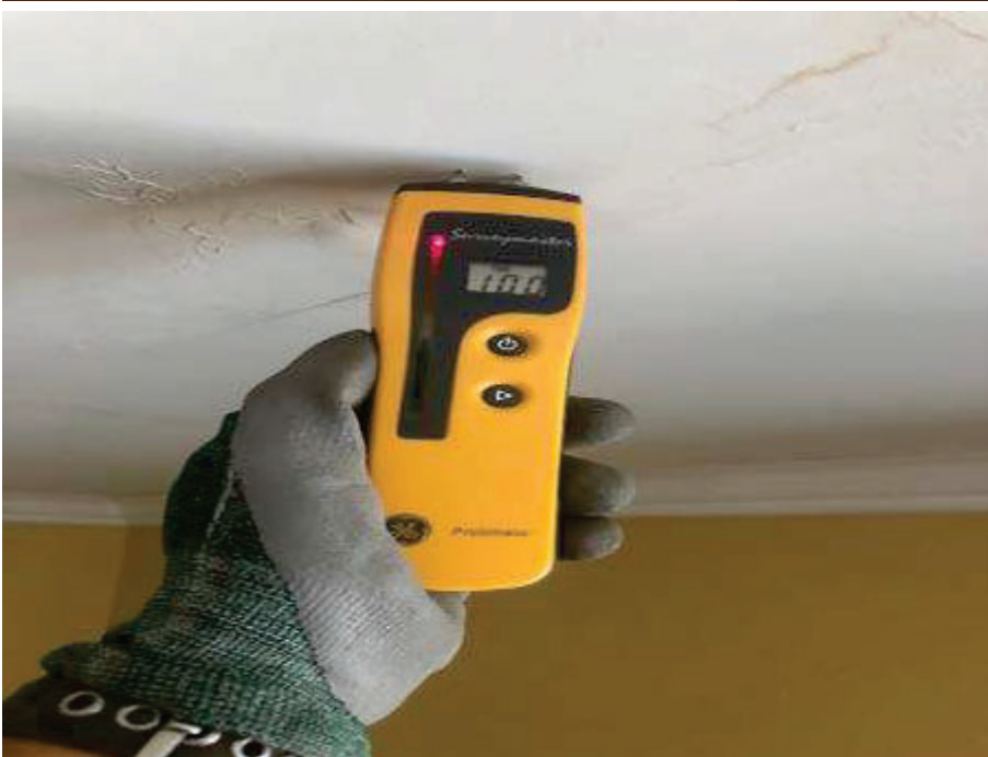
36. Marina Inn, Room 330 – View of elevated moisture readings on bedroom ceiling.
