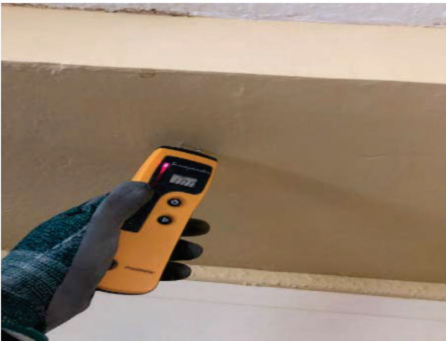
11. Marina Inn, Room 318 – View of elevated moisture reading on soffit.
