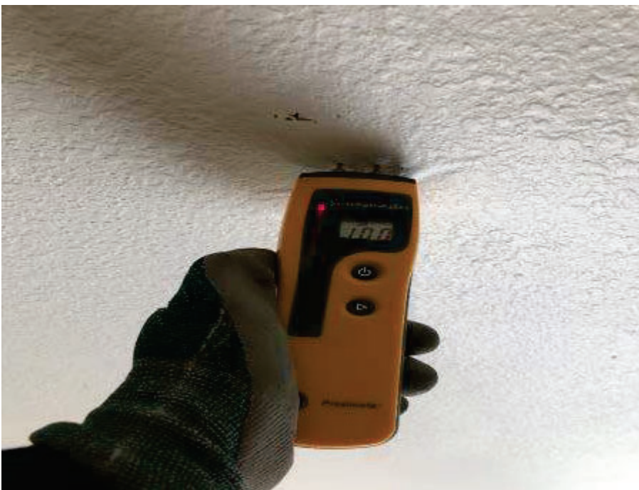
26. Marina Inn, Room 361, View of high moisture readings on bedroom ceiling.
