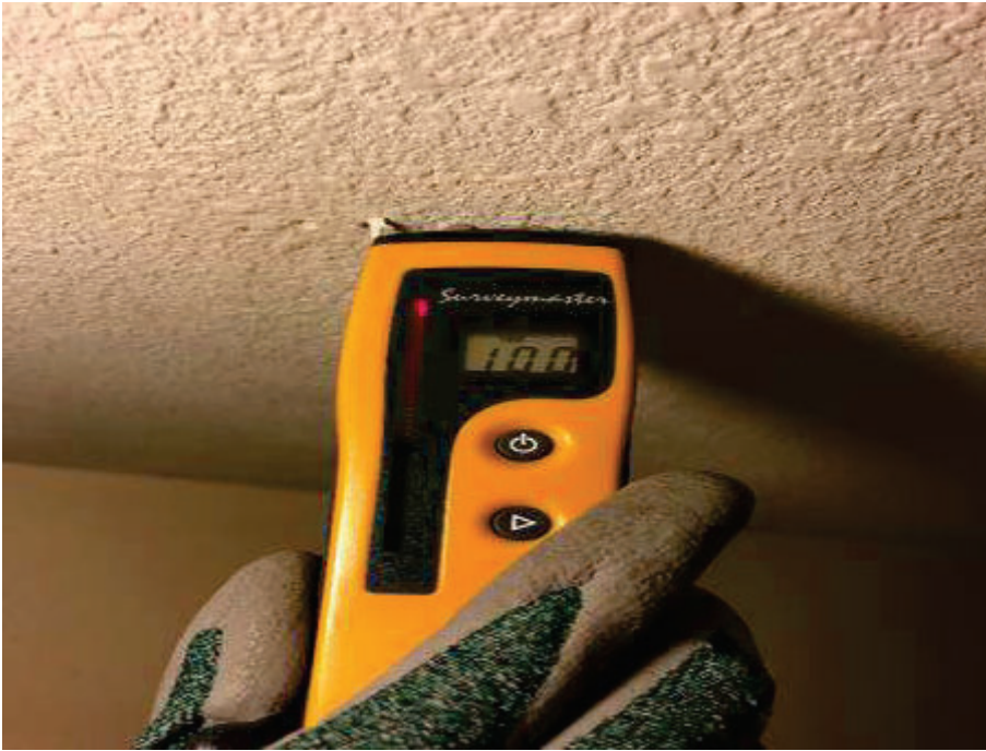
31. Marina Inn, Room T3 – View of high moisture readings on ceiling.
