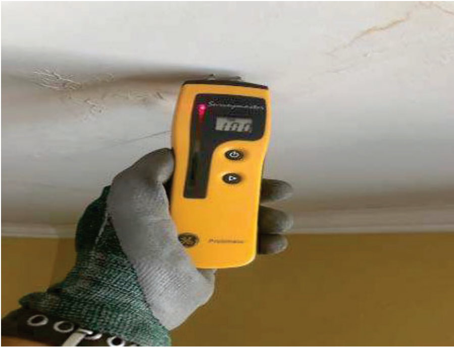
41. Marina Inn, Room 330 – View of elevated moisture readings on bedroom ceiling.
