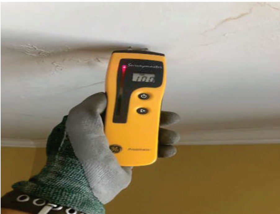
13. Marina Inn, Room 330 – View of elevated moisture readings on bedroom ceiling.
