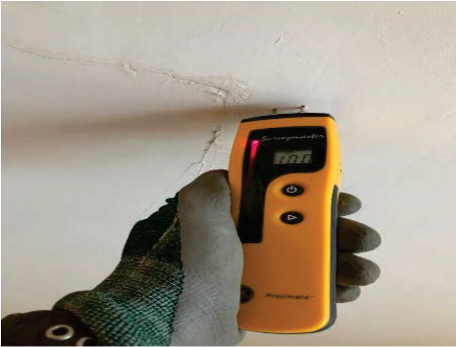
15. Marina Inn, Room 310 – View of elevated moisture readings on bedroom ceiling.
