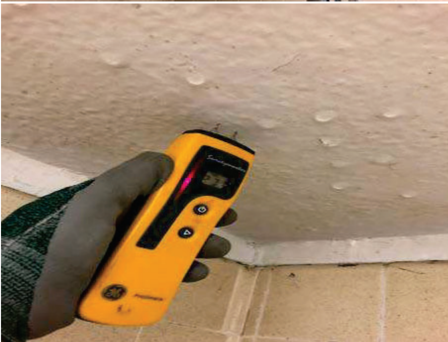
62. Building 4, Men's Restroom – View of elevated moisture readings and visible water condensation on ceiling above shower.
