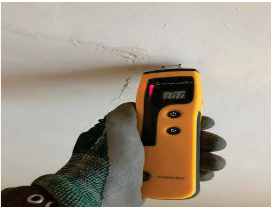
43. Marina Inn, Room 310 – View of elevated moisture readings on bedroom ceiling.
