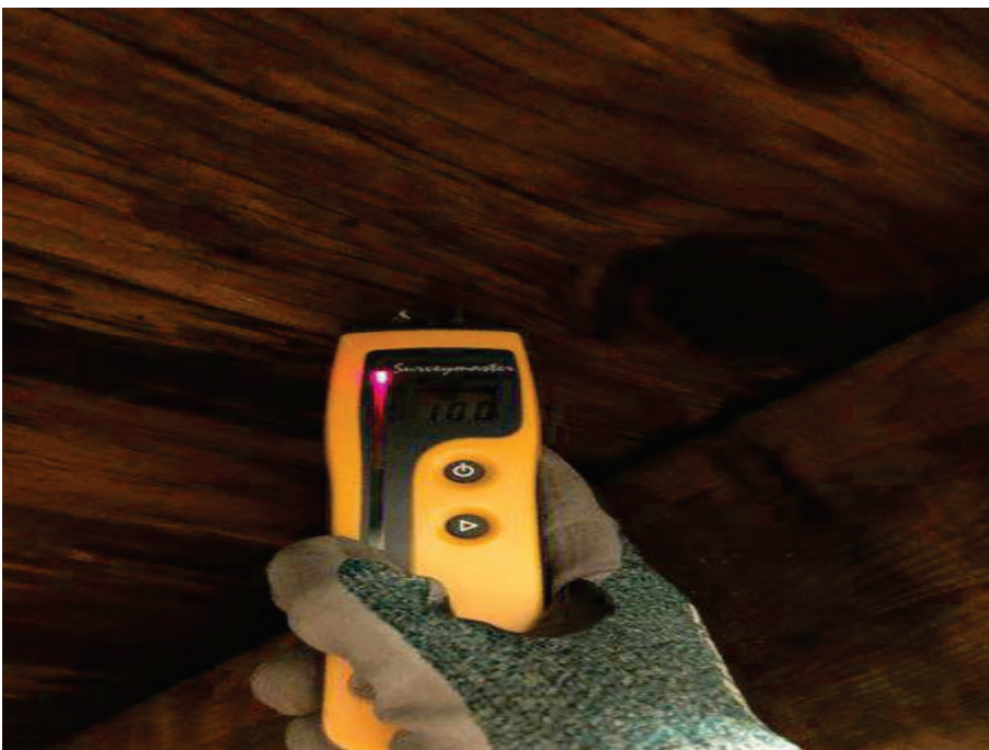
34. Marina Inn, Room 3D – View of elevated moisture reading.
