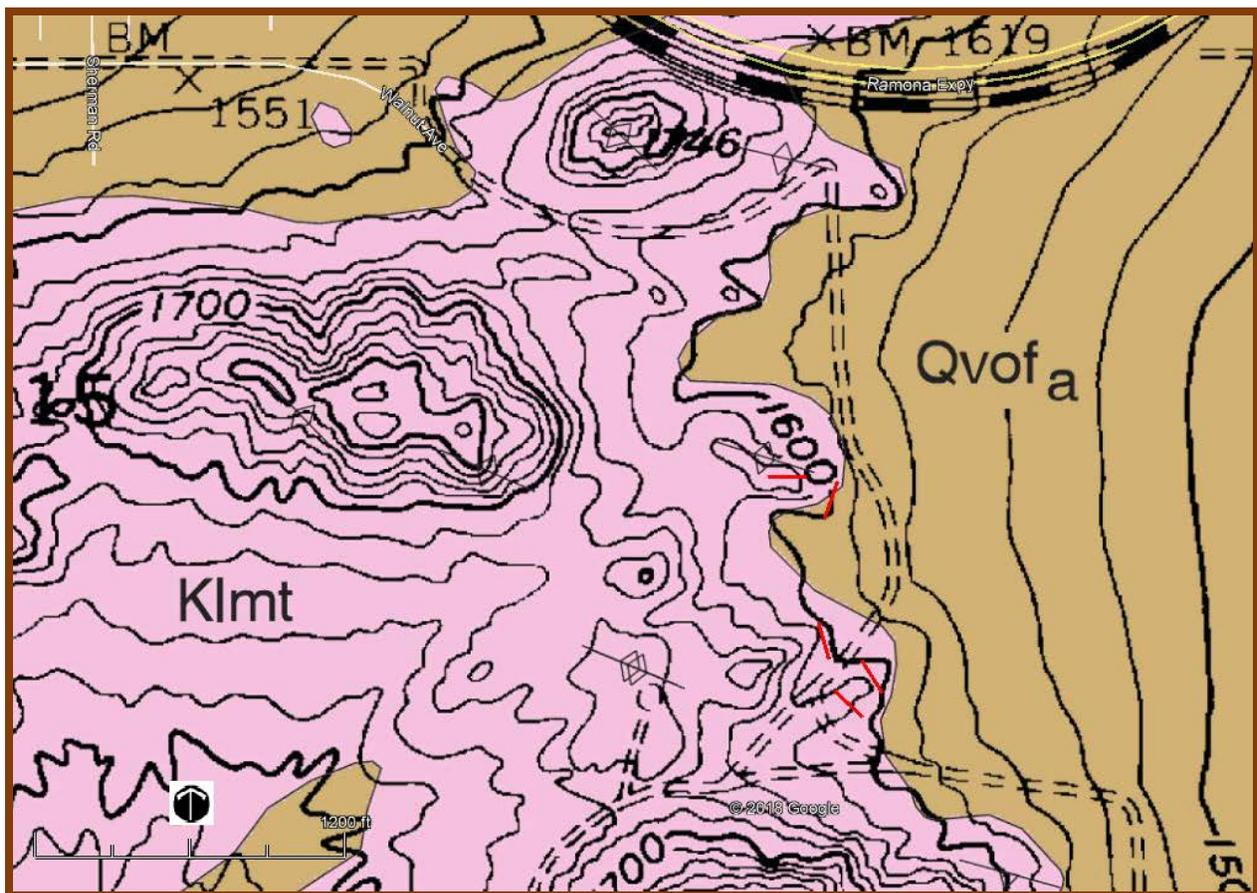
FIGURE 1- Geologic Map (Morton, 2003), Seismic traverses shown as red lines.
