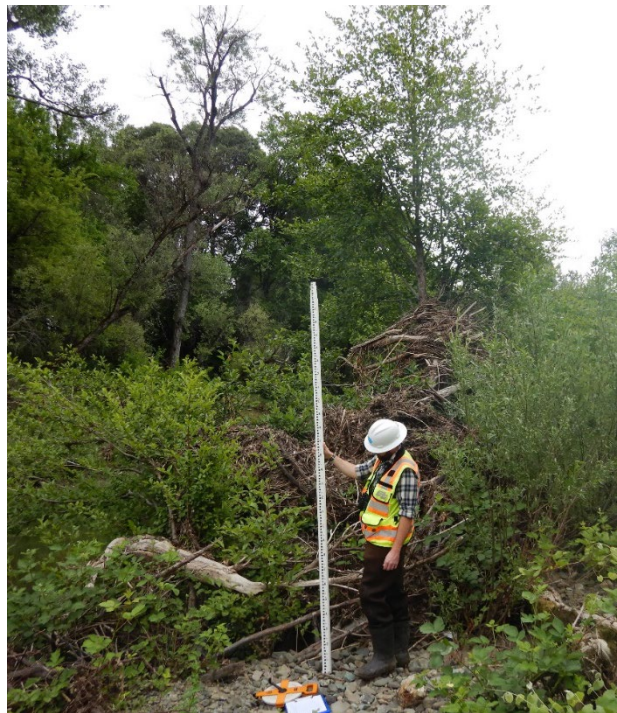
Photo 5: Image taken May 16, 2019 shows debris approximately three meters higher than the lateral channel west of the Russian River's active channel.
