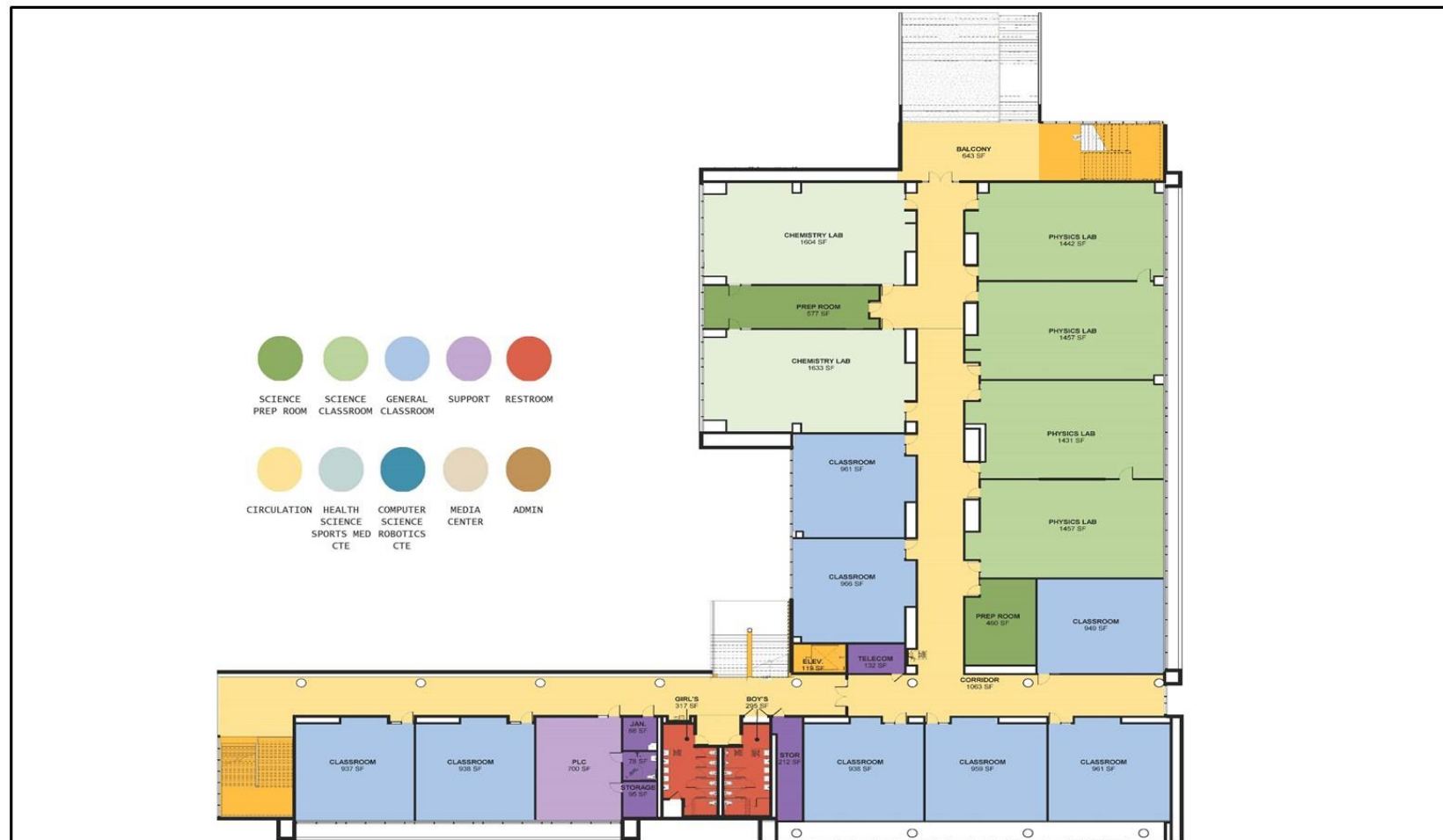
Figure 3.3-5 MULTISTORY STEM CLASSROOM BUILDING-SECOND FLOOR PLAN
