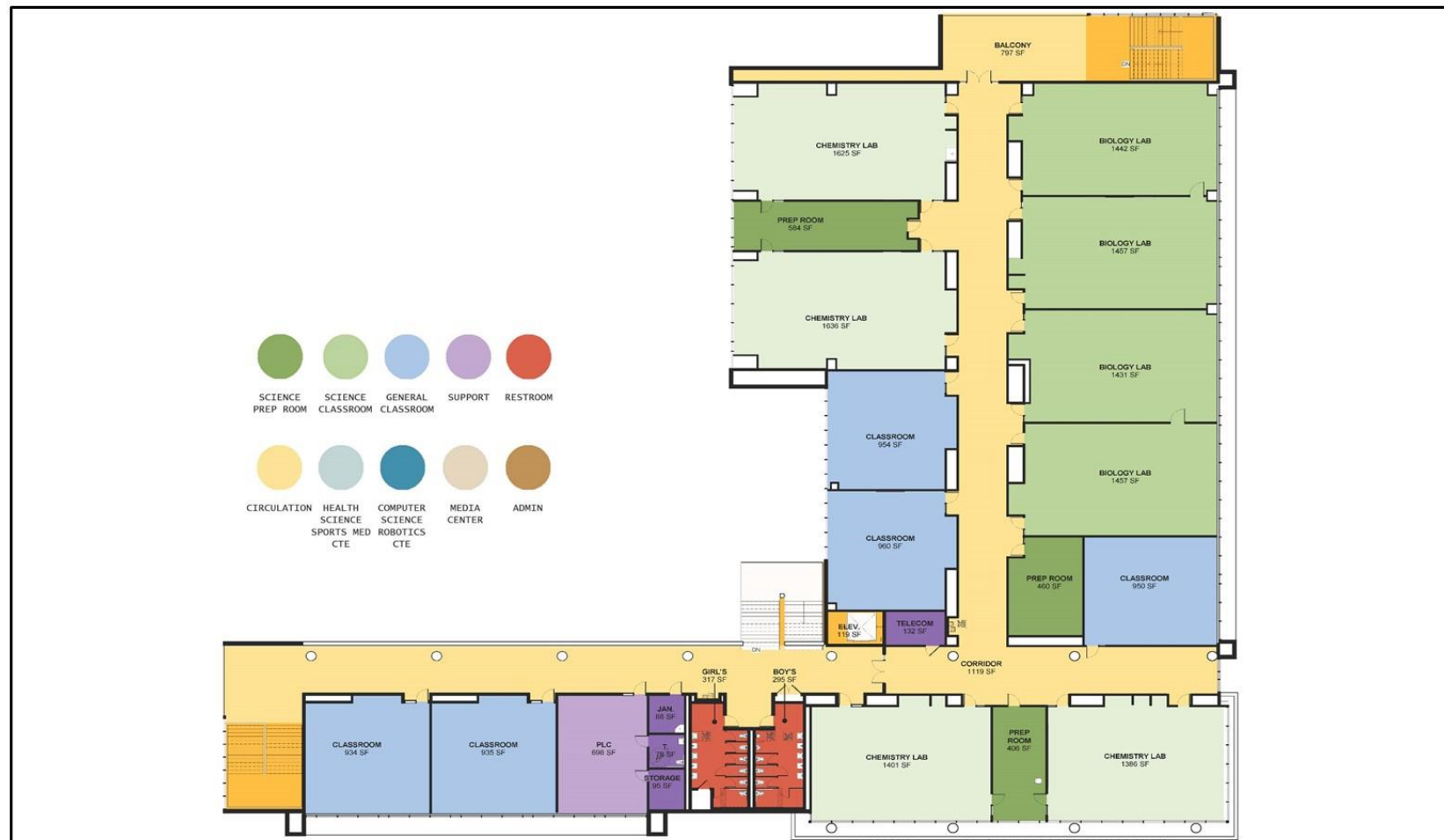
Figure 3.3-6 MULTISTORY STEM CLASSROOM BUILDING-THIRD FLOOR PLAN
