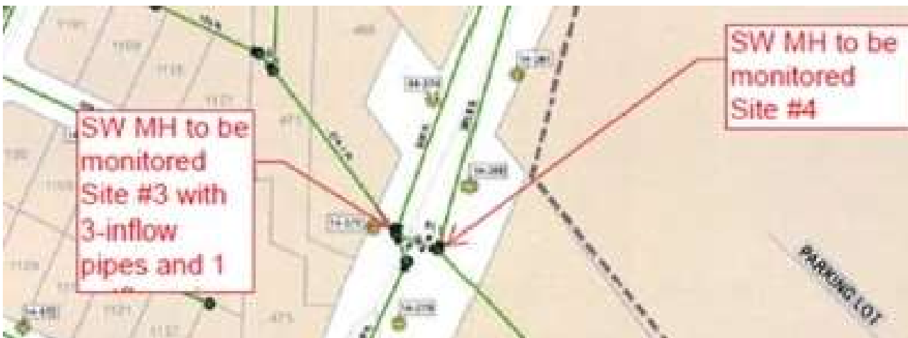
Figures: The vicinity map (above) shows the temporary wastewater flow monitoring locations of the Site 3A MH and the Site 3 MH. Site 3A MH is at latitude 33.909343 and longitude -117.889338 and Site 3 MH is at latitude 33.909322 and longitude -117.889302. The sewer map (below) shows the locations of Sites 3 and 4, which were incorrectly identified during the first week of monitoring.
