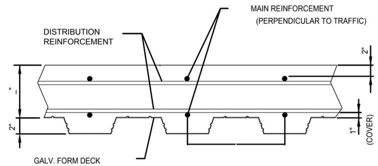
**4 CONCRETE DECK REINFORCEMENT**
