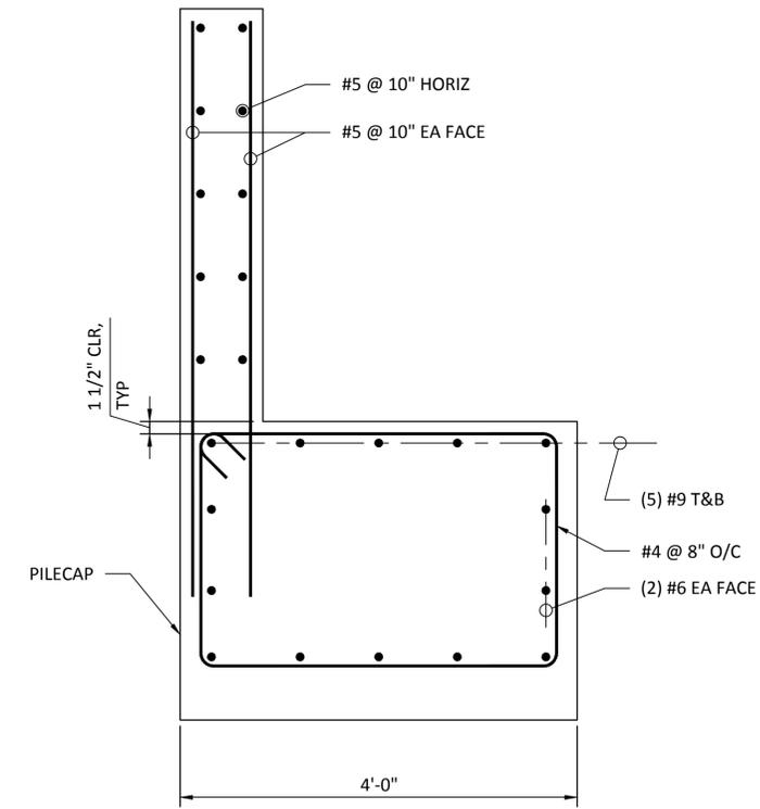
**3 TYPICAL BRIDGE ABUTMENT DETAIL**
