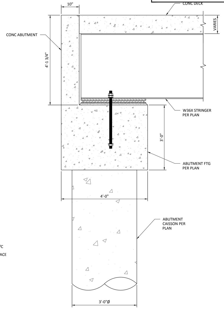
**4 TYPICAL BRIDGE ABUTMENT DETAIL**
