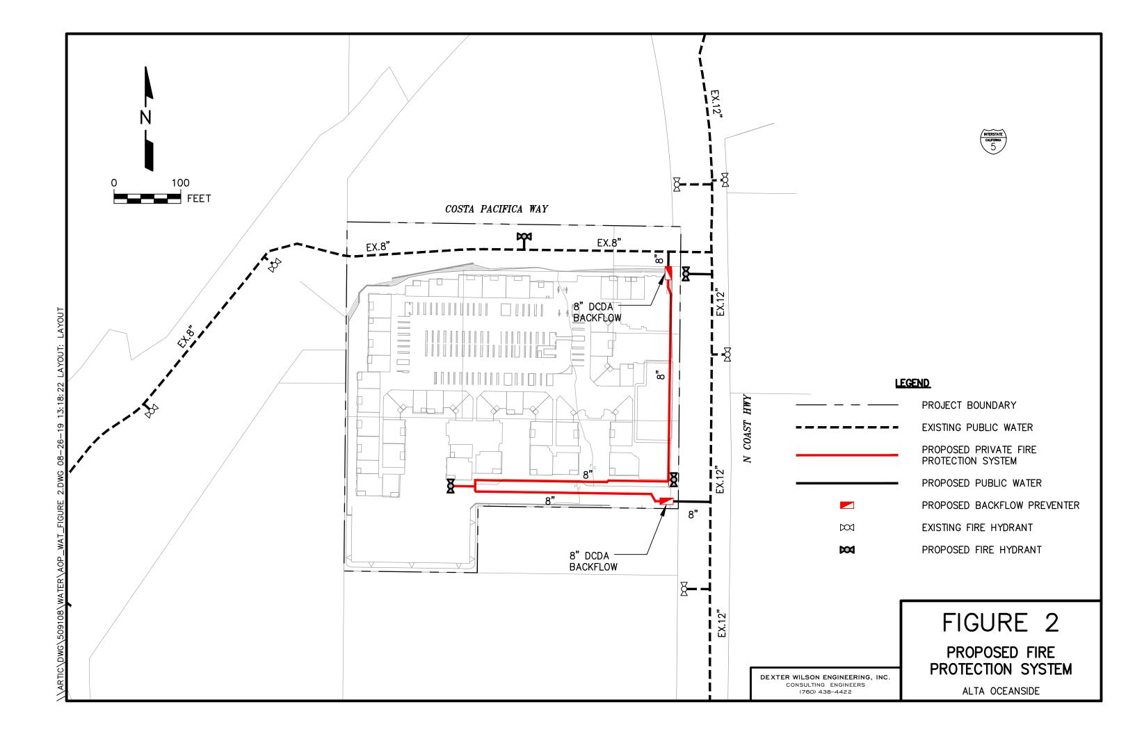
Water System Computer Model. Analysis using the KYPIPE computer software program developed by the University of Kentucky determined residual pressures throughout the water system. This computer software utilizes the Hazen-Williams equation for determining headloss in pipes. The Hazen-Williams "C" value used for all pipe sizes in our analysis is 120.
