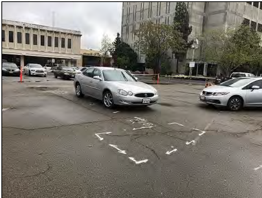
Photograph 2: Identified and delineated UST located in the area of the former garage.
