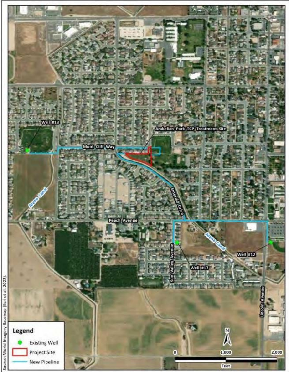
Figure 3 - Addendum No 1 Approved TCP Treatment Site at Arakelian Park and Associated Water Pipelines
