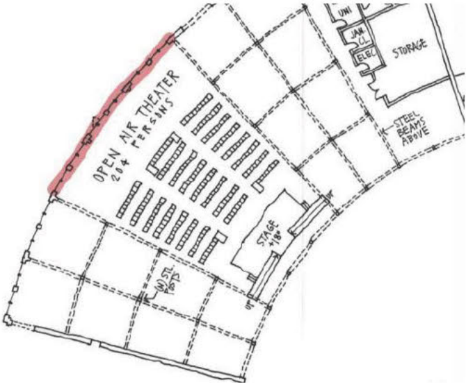
Figure 8: West half of proposed programming, 60-foot-long unbraced brick wall highlighted
