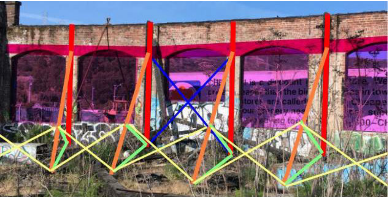
Figure 37: (below) Temporary shoring of brick walls.
