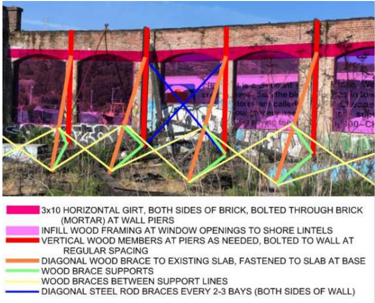
Figure 4: Temporary shoring of brick walls.
