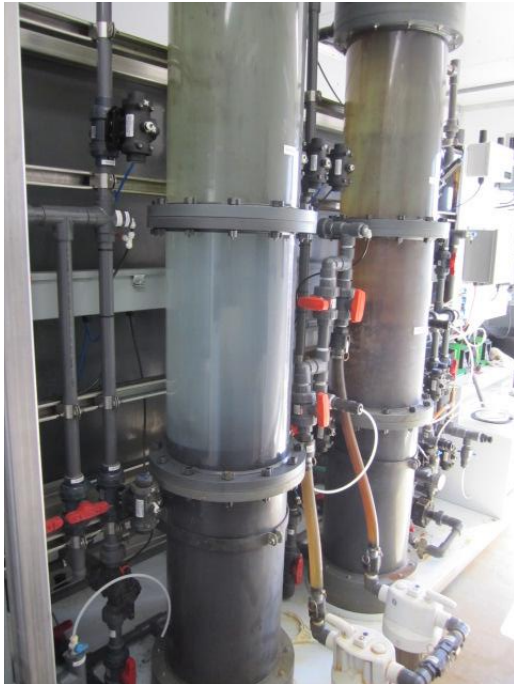
Photo 20. RCF Pilot System with zero valent iron columns
