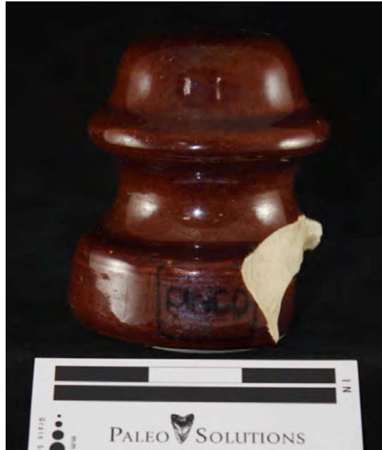
Brown porcelain insulator manufactured by The Porcelain Insulator Company. 20150929BCC.01H. Artifact #78
