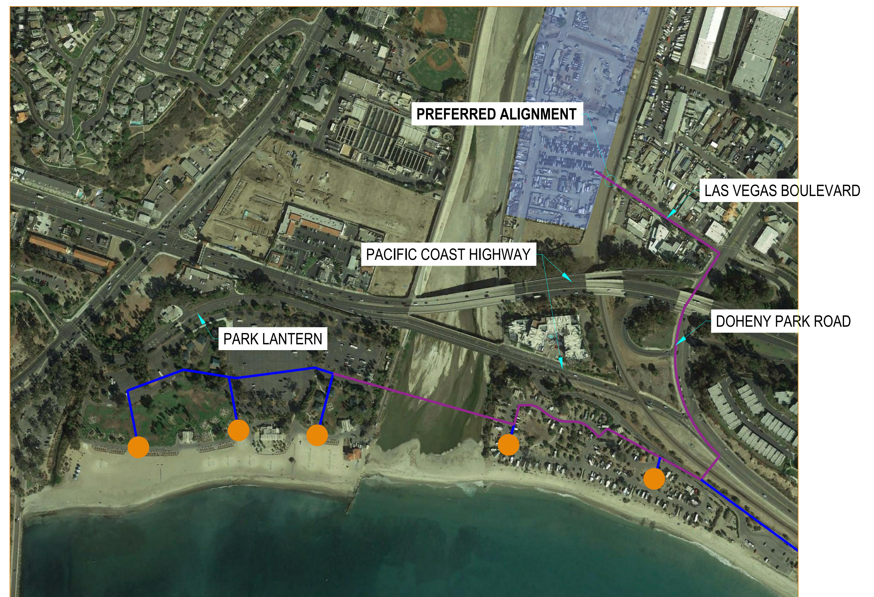
3 RAW WATER CONVEYANCE LAYOUT - PREFERRED ALIGNMENT 1" = 270'
