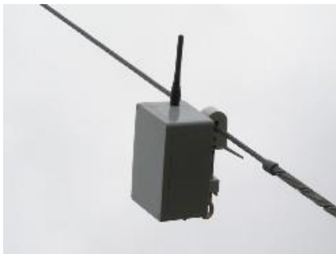
Figure 3.1 Bird Strike Indicator (BSI) attached to a power line. BSIs are relatively small devices that can be attached to a single wire of a power line and automatically register bird collisions based on the vibration of the wire.
