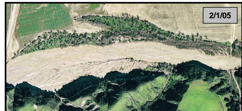
Figure 6. Progression of aerial photographs downstream of Castaic Canyon, showing channel change between 1993 and 2005. Note that there was little change between 2000 and 2004, but the active corridor widened significantly in response to the 2005 events, and that channel traces within the active corridor were effectively erased. See appendix A for photo sources.
